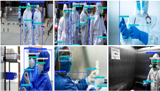
Fig. 3. Examples of model inference on test images showing PPE detection through bounding boxes and predicted classes.
