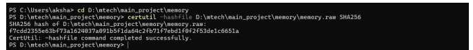
Fig. 3. Independent SHA-256 hash verification of the reconstructed memory.raw file using Windows certutil . The computed hash (f7cdd2355e63bf73a1624037a091b5f1da64c2fb71f7ebd1f0f2f53de1c6651a) matches the hash reported by Hiber2Bin in Figure 1, confirming that the reconstruction process preserved evidentiary integrity.
