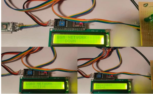
Figure 7: LCD display indicating GSM network unavailability and system status before LoRa mode activation, LCD display showing LoRa mode activation
