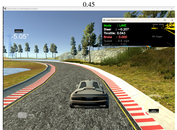
Fig. 4. Straight road tracking with both yellow lines detected
