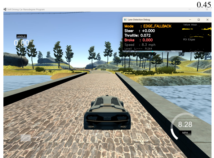
Fig. 4. Straight road tracking with both yellow lines detected
