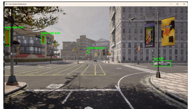
Fig. 7. Phase 2 qualitative results in the CARLA simulator. YOLOv8n detections are overlaid on the camera feed with colour-coded bounding boxes.
