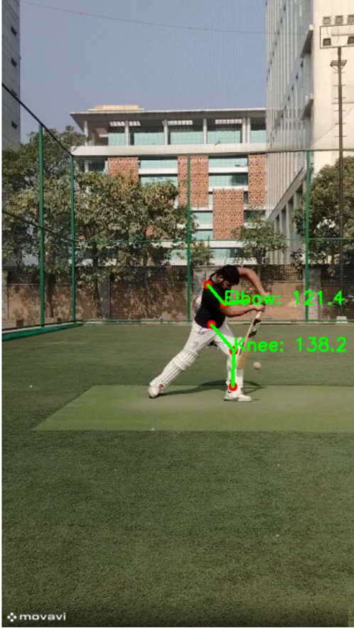
Fig. 6. Angle overlay visualization at the detected contact frame. Elbow and knee angles are superimposed on the player's posture to validate biomechanical metric computation.
