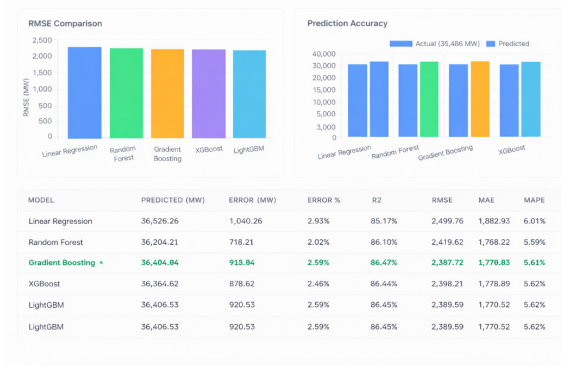
Fig. 7. Model Comparison page showing side-by-side R^2 , RMSE, and prediction accuracy for all five models.
