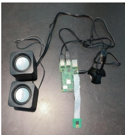
Fig. 6. Physical Hardware Setup of the Prototype Kiosk
