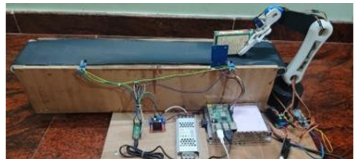
Fig.4 RFID scanning process after the package reaches the second IR sensor.
