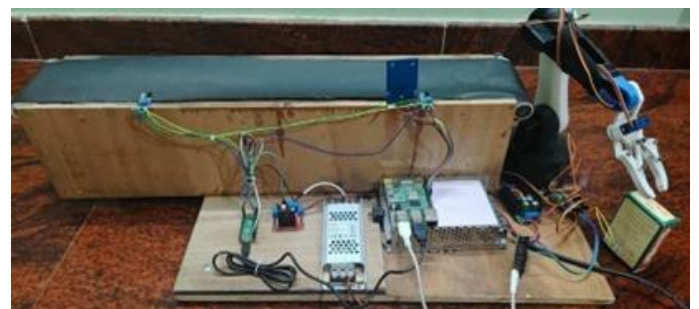
Fig.5 Robotic arm performing pick-and-place operation into designated bins.
