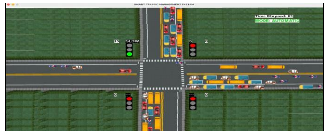
Fig. 6: Annotated frame showing lane-wise vehicle detection, counts, and density [10].
