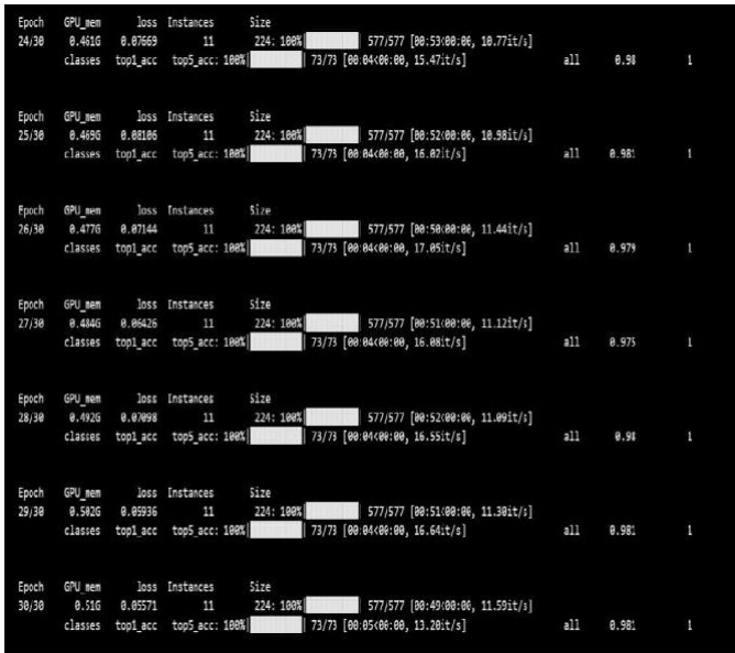
Figure3: Training Progress of CNN Model Showing Epoch-wise Loss, Accuracy, and GPU Utilization
