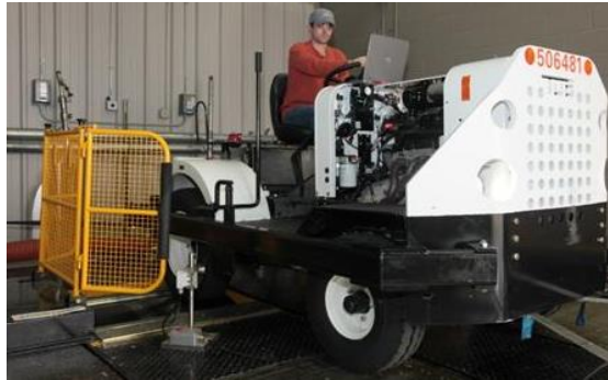
Fig. 9: Chassis dynamometer test setup
