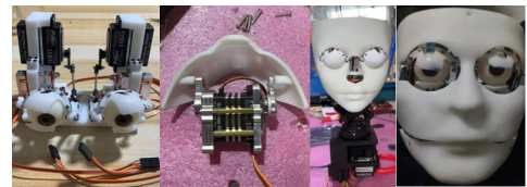
Fig. 8. Process of Robot Headshell and Silicone Fabrication.
